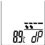
The dew point temperature is the point the temperature must drop below for the air to precipitate its water vapour in the form of droplets, mist or dew. Condensation water therefore occurs for example when the temperature of an inside wall or window reveal is lower than the dew point temperature of the room. These areas are then damp and are a breeding ground for mildew/mould with possible material damage.
