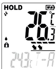
Display of infrared temperature (in all measuring modes)
