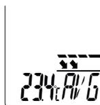
Max/Min/AVG modes refer to the infrared temperature and show the maximum, minimum or average infrared temperature. With the trigger (9) pressed, the Max/Min/AVG values are determined while measuring. The value is deleted and calculated again at the start of a new measurement or by pressing the trigger (9).
