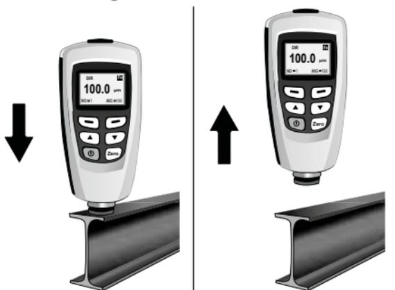
**!** During measurement, keep the device as straight, tangential and still as possible.
