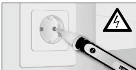
If voltage is present, the detector tip lights up and a signal sounds.
