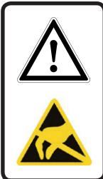
The enclosure is constructed from plastic. To prevent the risk of electrostatic sparking the plastic surface should only be cleaned with a damp cloth.
