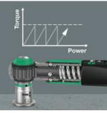
The Safe-Torque A 1 torque wrench is equipped with a slideover mechanism. Once the set torque value has been reached, the tool cannot be overtightened, so that excessive torque cannot be applied.
